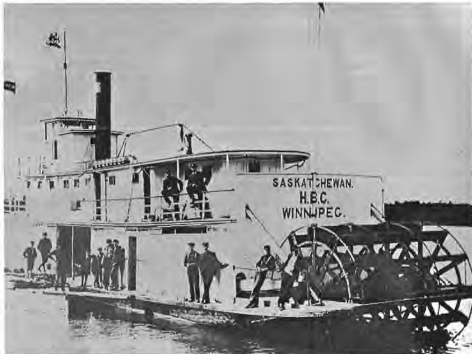
This photo could well be captioned "Hands to stations for leaving harbour" as the old river steamer Saskatchewan leaves Squaw Rapids, on the Saskatchewan River, for Cumberland House, sometime before the turn of the century. The 146-foot stern wheeler is believed to have been the first ship in Canada named Saskatchewan. (E-78353)
