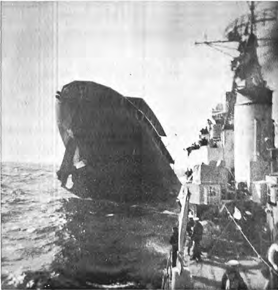
The Athabaskan approaches the stern section of the tank Amphiclos, which broke in two in the North Atlantic on March 1, 1964. (HS-74376)
