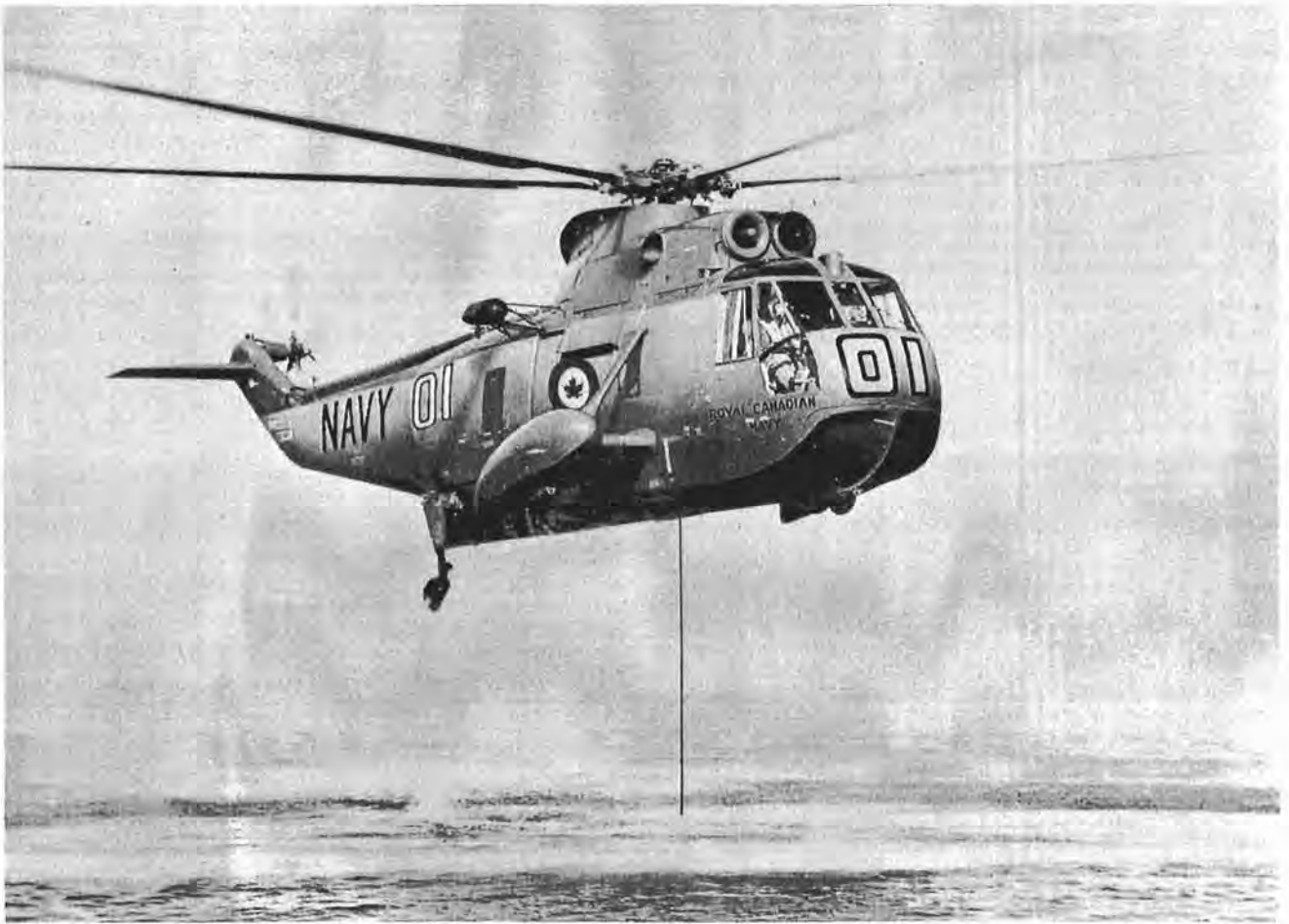
The first Sikorsky CHSS-2 twin-turbine all-weather helicopters will be delivered to the RCN in May. Nine of these helicopters are being obtained during the 1963-64 fiscal year. Each will carry a crew of four, two pilots and two sonar operators. Equipped with the latest navigation, detection and weapon systems, the CHSS-2 will be capable of locating, tracking and attacking a submarine while operating in conjunction with or independently of surface ships. (CN-6572)
