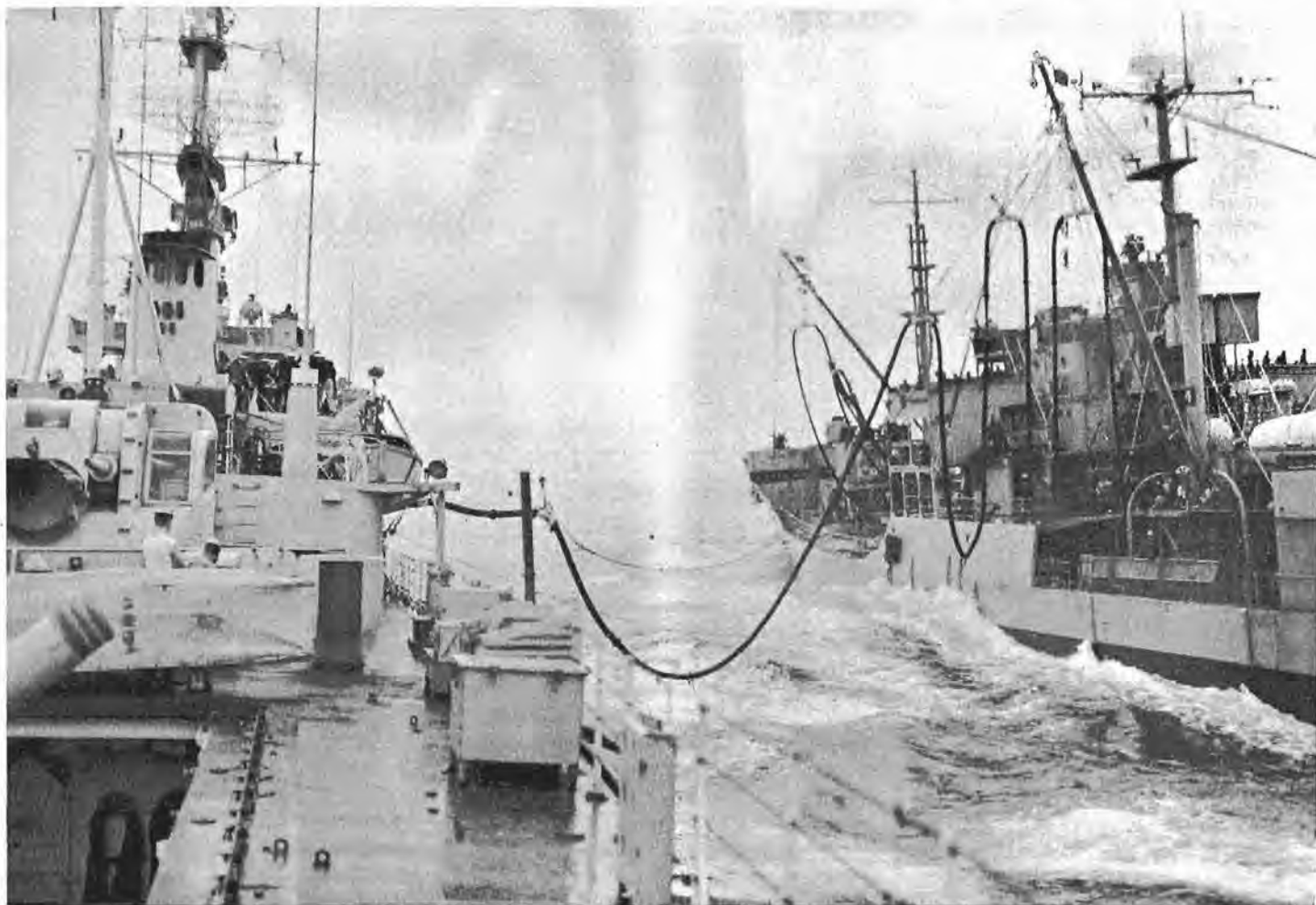
HMCS Restigouche fuels from a U.S. Navy tanker during NATO fleet manoeuvres in the Atlantic. Standard hose couplings are fitted in NATO ships. (HS-64756-70)
