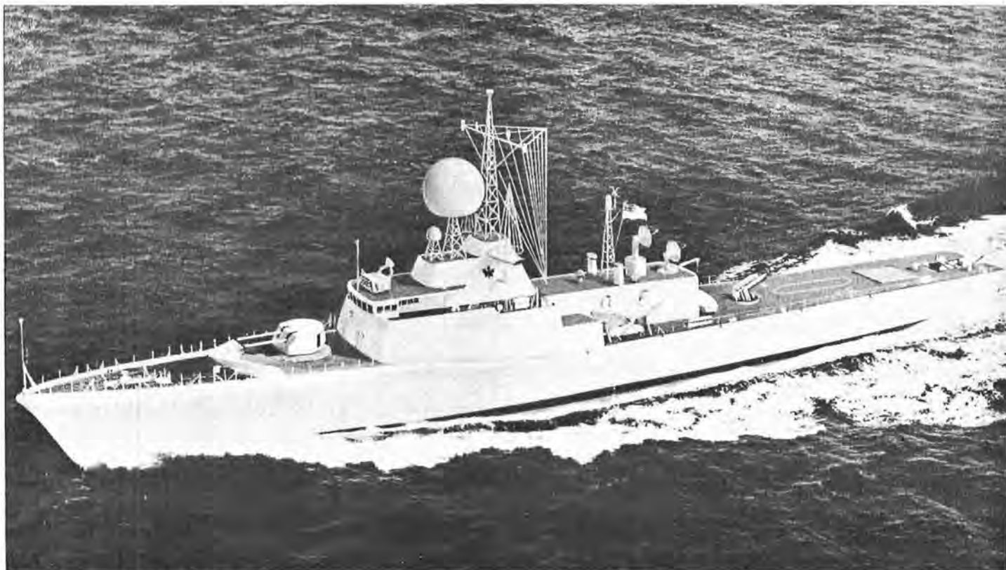
This is an artist's conception of the proposed General Purpose Frigate. Construction on the first of eight of these frigates will begin in 1964 and all are scheduled for completion by 1970. The ships will carry two missile systems for anti-aircraft and anti-missile defence and will be fully equipped with anti-submarine detection and attack facilities. Armament will include a twin five-inch gun mount. The ships will be capable of transporting a company of combat troops, complete with equipment, landing them and supporting operations ashore. A utility helicopter, carried on board, will be of tactical value to Army operations ashore. (CN-6523)
