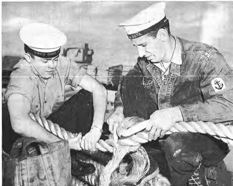
Engrossed in making an eye-splice in a six-inch hawser are Ord. Sea. Jerry G. Howe (left) and Ldg. Sea. Pelham P. Young. They serve in the destroyer escort Terra Nova , based at Halifax. (HS-70380-14)
