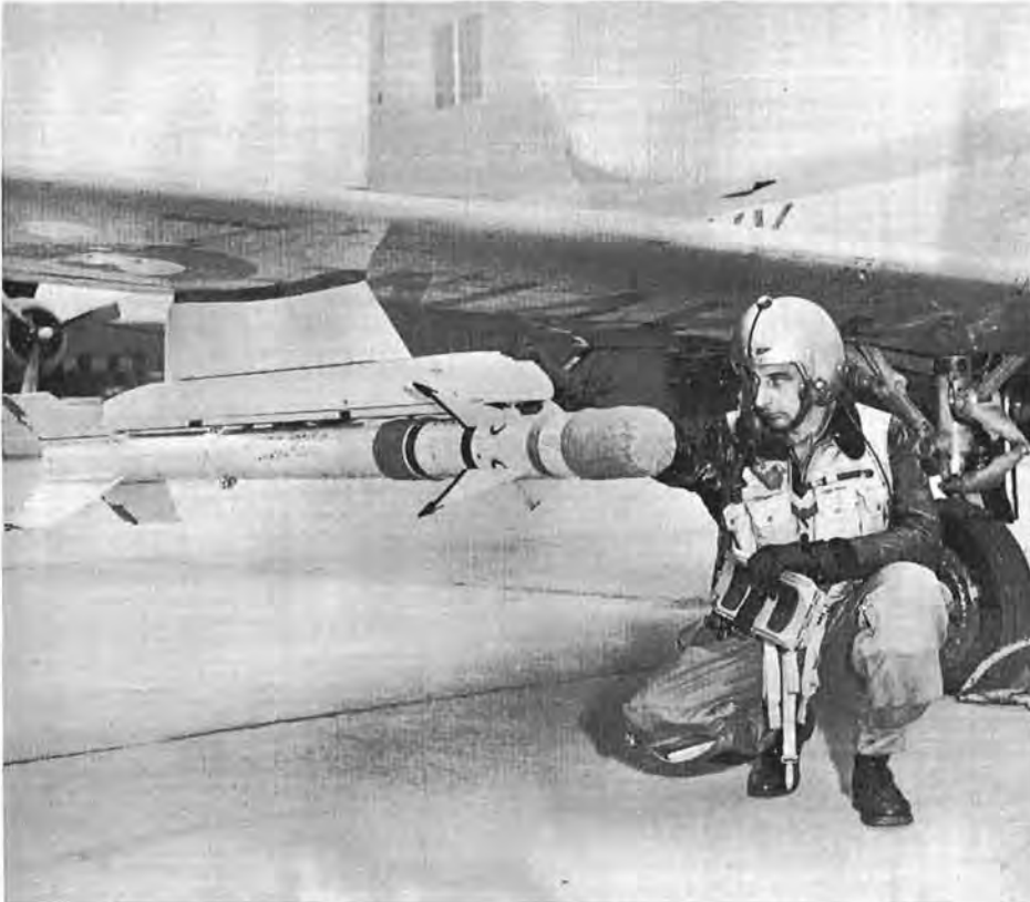
The Royal Canadian Navy in 1958 became the first of Canada's armed forces to arm itself with guided missiles. A Sidewinder is shown slung beneath the wing of a Banshee jet fighter. (DNS-21044)
