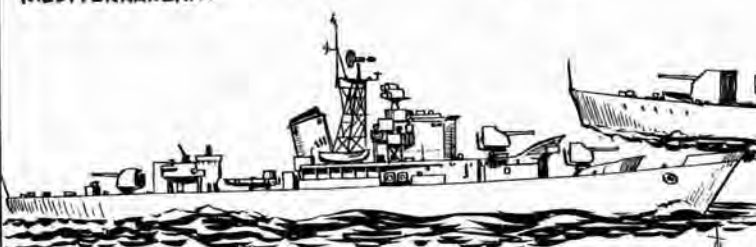
RUSSIAN 'RIGA' CLASS FRIGATE (900 TONS). THREE 3.9 IN. GUNS. APPEAR TO BE SMALL DESTROYERS...
