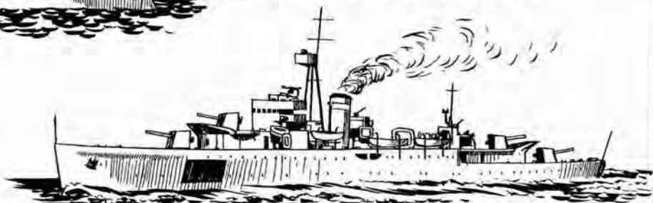
PORTUGUESE SLOOP 'BARTOLOMEU DIAS' - BUILT IN BRITAIN, DESIGNED FOR COLONIAL SERVICE - 4 4.7 IN. GUNS AND 40 MINES. FORMERLY CARRIED 1 SEAPLANE.
