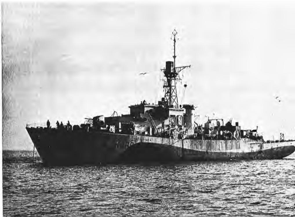
As the Second World War progressed, the urgency of building staying-power into warships was realized. The Revised Single-Screw (Increased Endurance) corvette was one answer. Others were the frigate (originally styled "super-corvette") and the Castle class corvette, such as HMCS Hespeler, shown above, which was armed with squid. (A-389)
