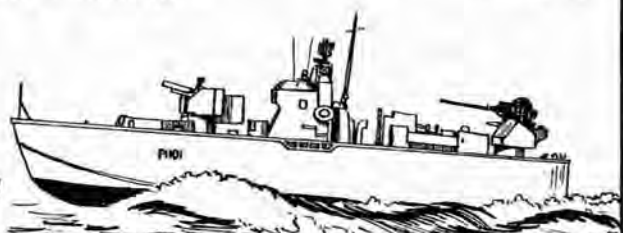
BRITISH 'DARK' CLASS CONVERTIBLE MOTOR TORPEDO/MOTOR GUNBOATS (DELTAIC ENGINES). AS GUNBOATS THEY CARRY 1 4.5 IN. GUN, AND 1 40 MM A.A. GUN. AS M.T.B.s THEY CARRY 4 21 IN. TORPEDO TUBES AND ONE 40 MM A.A. GUN. SPEED IS APPROXIMATELY 40 KNOTS.
