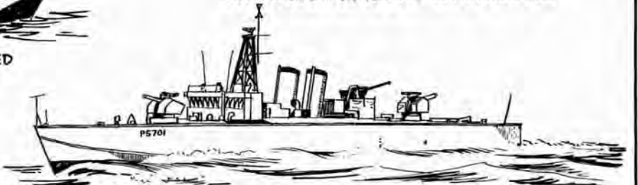
H.M.S. BOLD PIONEER—FAST PATROL BOAT... (GAS-TURBINE). AS A GUNBOAT SHE MOUNTS 2 4.5 IN. GUNS & 1 40 MM A.A. AS A TORPEDO BOAT SHE IS ARMED WITH 4 21 IN. TORPEDO TUBES AND 1 40 MM A.A.
