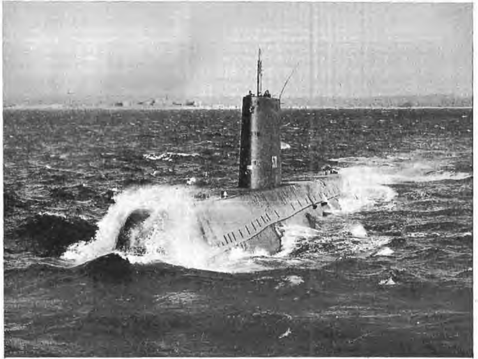
During the first year of service the nuclear-powered U.S. Submarine Nautilus steamed 60,120 miles without replenishing her fuel. The New York Times estimated that if the Nautilus had been diesel-powered she would have consumed 720,000 gallons of oil during her journeying. Once again warships have attained the freedom from reliance on fuelling bases enjoyed during the great days of sail. (Official United States Navy Photograph)
