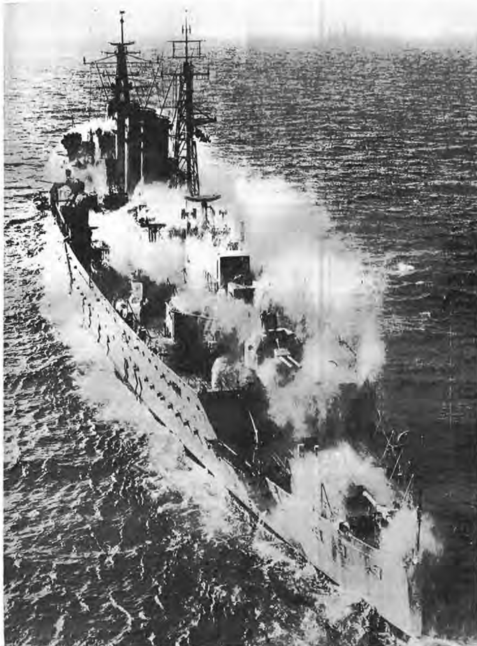
The Royal Navy's trials cruiser Cumberland is seen as she carried out anti-atomic tests in the Mediterranean. A harmless quantity of radioactive liquid was scattered over her decks and then the hosing-down equipment was turned on to test its efficiency. The results showed that atomic fission matter could be quickly removed by such a washdown, with the ship's company below decks out of harm's way. (Photo courtesy U.K. Information Office.)
