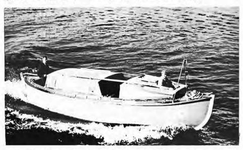
The 27-foot Canadian motor sea boat is shown going through its paces at the Amprior "regatta". This boat is a modification of the Royal Navy motor seaboat, the main difference being a whaler stern, greater power and omission of the mast and sails. (O-6008)
