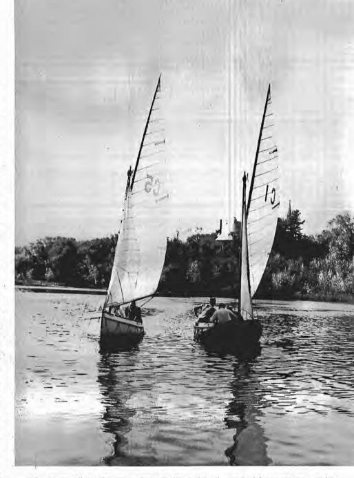
Crows compare the performances of two dinghies under sail. On the left is a prototype 14-foot dinghy built of polyester resin reinforced with fiberglas cloth and mats. It is the first boat of this type of construction to be built for the RCN. (O-6014)
