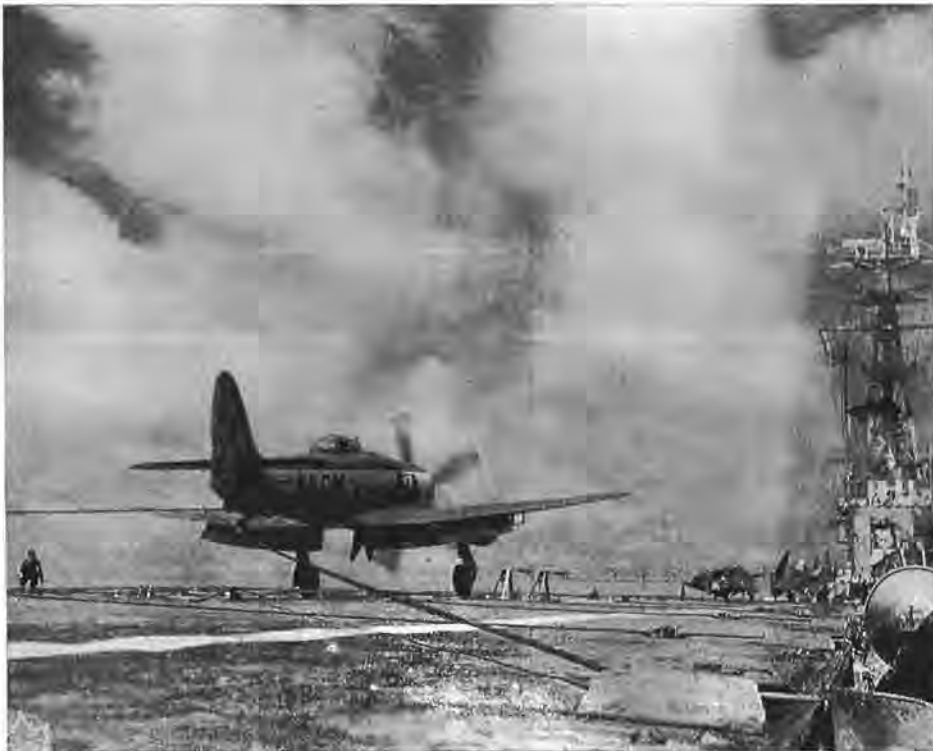
A Sea Fury of 871 Squadron catches an arrestor wire in landing on the flight deck of the Magnificent during flying exercises in which the aircraft of 30 Carrier Air group spent 1,016 hours in the air in the month of August — a new record in the RCN. (MAG-3256).
