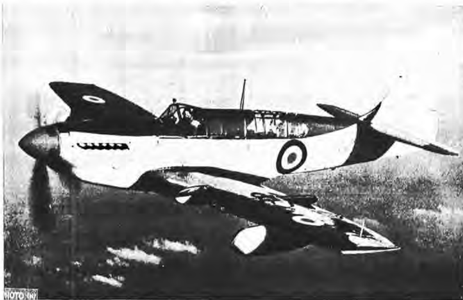
This is the Firefly V with which 825 Squadron, now in the United Kingdom, is being equipped. The squadron will return to Canada February 23 on board H.M.C.S. "Magnificent". An all-metal, two-seat monoplane, the Firefly V is powered by a Rolls Royce Griffon engine. It is equipped with four 20-mm. cannon, radar and radio installations, and the latest airborne anti-submarine devices.
